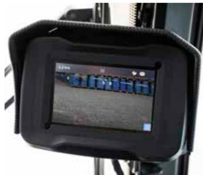
The jog shuttle-controlled LCD screen displays critical updates and automatically switches to the rear-view camera's feed when in reverse.
