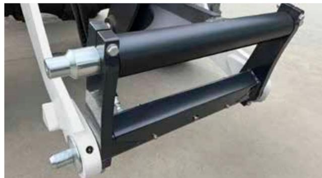
Quick-Tach™ coupler (installed as standard)
