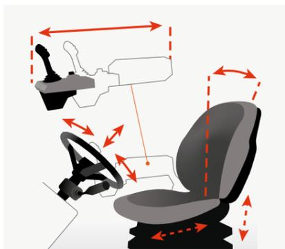
Easily adjust the position of the steering wheel, joystick and seat to what suits you best. Make your loader fit you like a glove.
